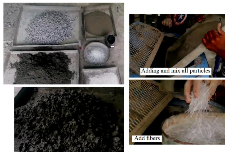
Fig. 1. Mix processing of cement, aggregates, and fibers.
