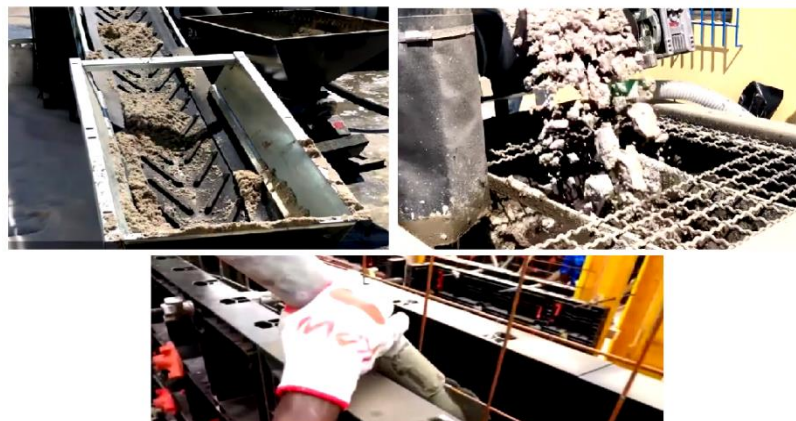
Fig. 1. A mixture of cement, sand, water, and foam.
