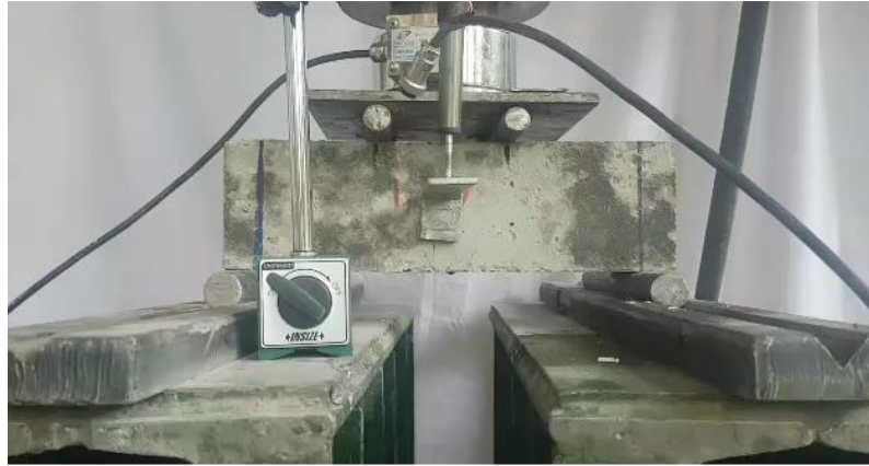
Fig. 10. Loading configuration for the flexural strength test.
