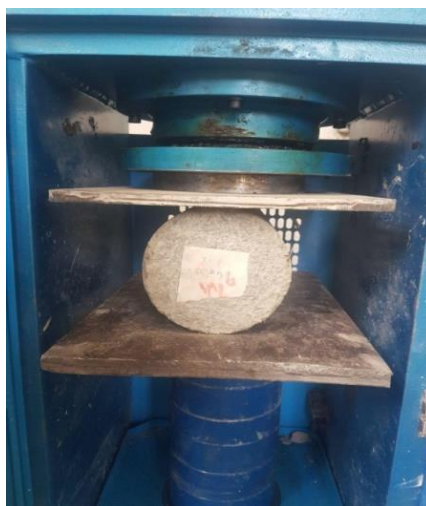
Fig. 9. Arrangement of the concrete specimen and loading strips between the loading platens of the testing machine for the Brazilian splitting tensile strength test.
