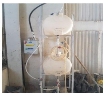
Fig. 6. Magnetized water generation device.
