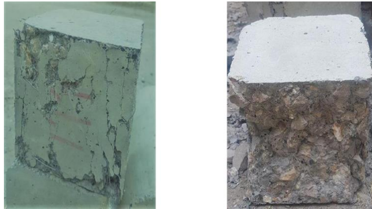
Fig. 12. Failure modes of compressive strength specimens: a. without steel fibers, and b. with steel fibers.
