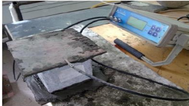
Fig. 8. Electrical resistivity measurement device.
