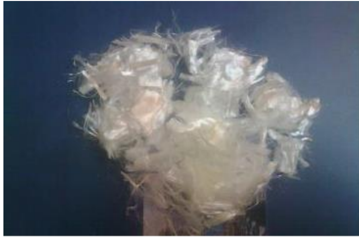
Fig. 2. Polypropylene fibers used in the experimental program.
