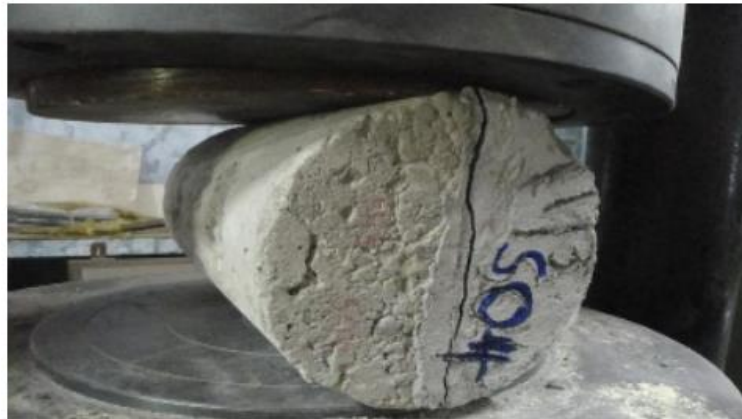
Fig. 4. Concrete specimen in the testing machine.
