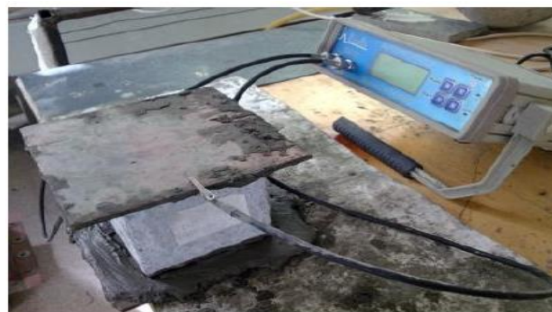
Fig. 8. Electrical resistivity measurement device.
