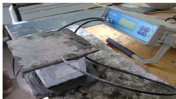
Fig. 8. Electrical resistivity measurement device.
