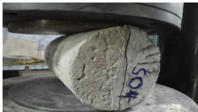
Fig. 4. Concrete Specimen in the testing machine.
