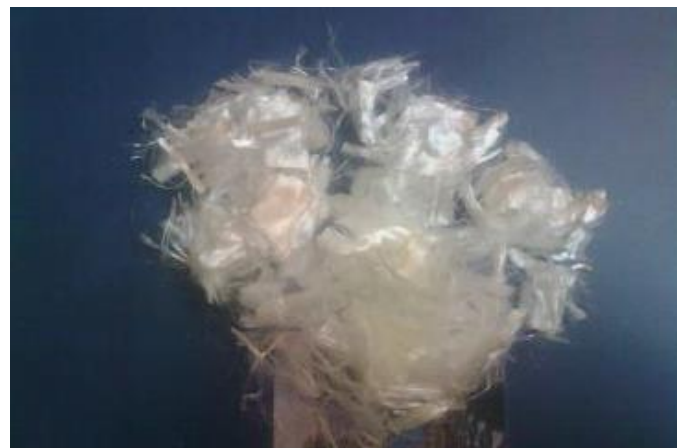
Fig. 2. Polypropylene fibers used in the experiments.
